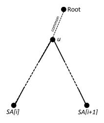
Then compute LCP(i, j) for any  $j \ge (i + 2)$  using the following **FACT**:  $LCP(i, j) = \min_{k=i}^{j-1} LCP(k, k+1)$ **Proof:**  $LCP(i,j) \le LCP(k,k+1) \forall k = i \cdots j - 1$   $\rightarrow LCP(i,j) \le \min_{k=i}^{j-1} LCP(k,k+1).$
