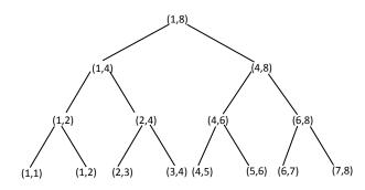
We have a complete binary tree with (1, m) as the root. Any internal node (i, j) will have two children  $(i, \lfloor \frac{i+j}{2} \rfloor) \& (\lfloor \frac{i+j}{2} \rfloor, j)$ There are *m* leaves  $(1, 1), (1, 2), (2, 3), (3, 4), \dots, (m - 1, m).$
