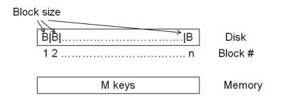
To begin with, there are N! permutations such that the correct answer could be any one of these. The number of permutations that can be generated in one I/O is  $\binom{M}{B}B!$ .
