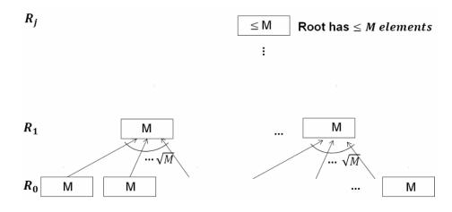
Think of a tree where the degree is  $\sqrt{M}$  and each leaf has M elements. First we sort each leaf and every leaf sends its keys with ranks  $\sqrt{M}, 2\sqrt{M}, ..., M$  to its parent. We continue this process in every node until we reach a node that has  $\leq M$  elements. This node is the Root. The leaves are at level 0 and let the level of the root be j.
