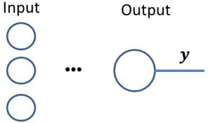
Let y be the expected output, and let  $y_a$  be the observed output. Adjust the weights proportional to the difference between y and  $y_a$ .
